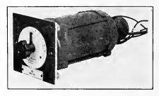
A color master of the Selsyn Thyratron light control equipment developed by General Electric
